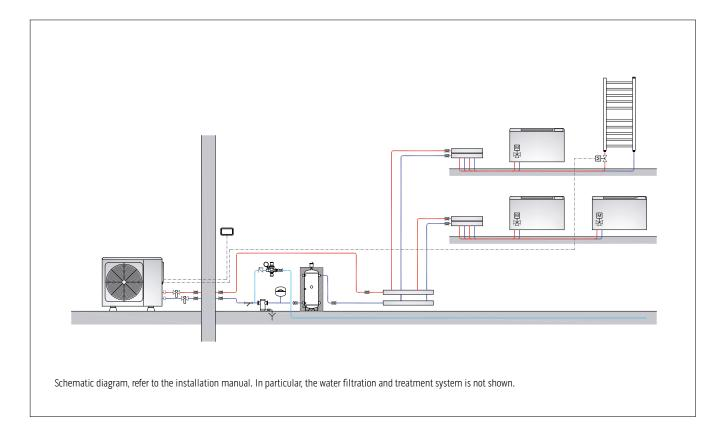
SHERPA MONOBLOC S2 E heat pump (heating and air conditioning; DHW production) Bi2 SLR radiant fan coil units, domestic water integration with solar thermal and integrated inertial storage (used as hydraulic separator) for the air conditioning system.
