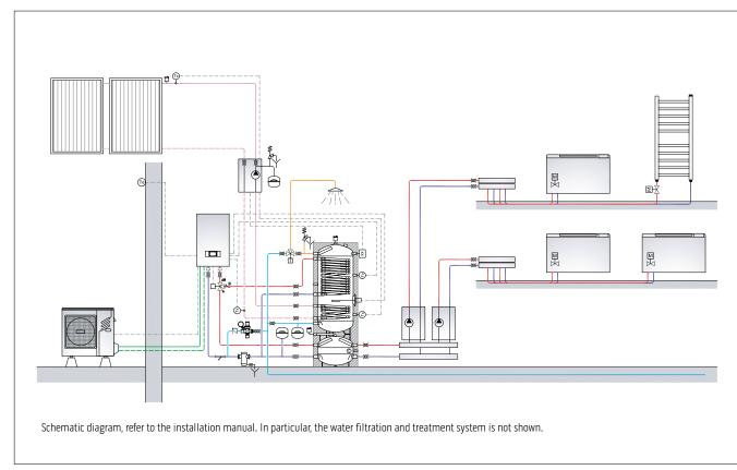
SHERPA TOWER S2/S3 heat pump (heating and air conditioning; DHW production) Bi2 SLR radiant fan coil units with 3-way valves and inertial storage in series on the return pipe of the air conditioning system.
