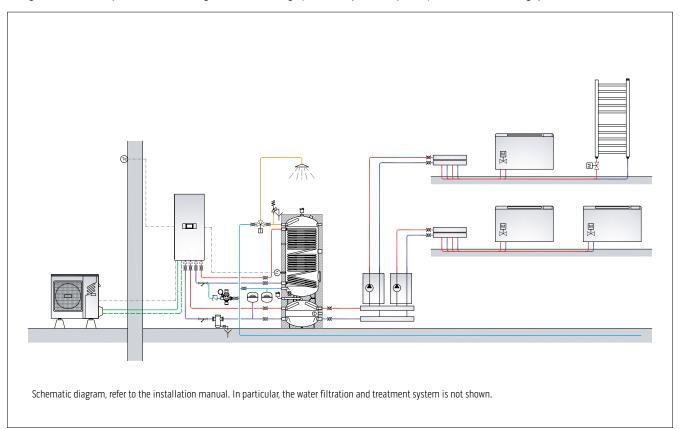
SHERPA AQUADUE TOWER S2/S3 heat pump (heating and air conditioning; production of high temperature DHW); Bi2 SLR radiant fan coil units; example of a two-zone configuration with a simple manifold and inertial storage (used as a hydraulic separator) for the air conditioning system.
